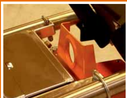
One centralized and balanced lifting eye.
