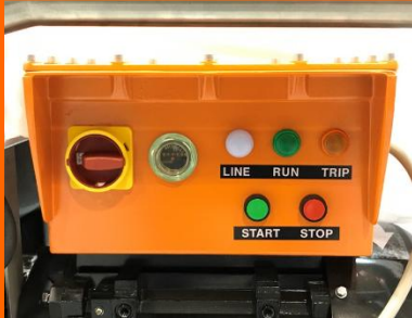
Electrical box with main switch, overload relay & hour meter.
